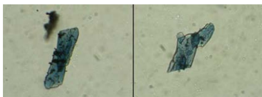
Figure 1. Optical microscopy pictures of complex 1 in the crystalline form showing the dark-blue thin plate crystals. Magnification: microscope \times 20 ; camera \times 3.8 .
